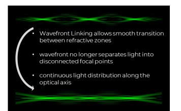
**Figure 2:** Wavefront Linking uses special linking zones to create a continuous distribution of light along the optical axis.
