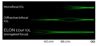
**Figure 3:** Simulated through-focus point spread functions for a monofocal, diffractive bifocal, and the ELON EDOF IOL, which creates a single elongated focus.
